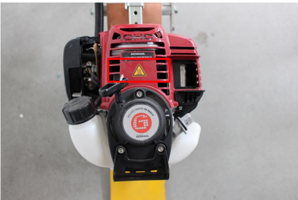
Figure 5: Installation positions for safety signs 3
