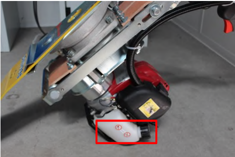
Figure 4: Installation positions for safety signs 2
