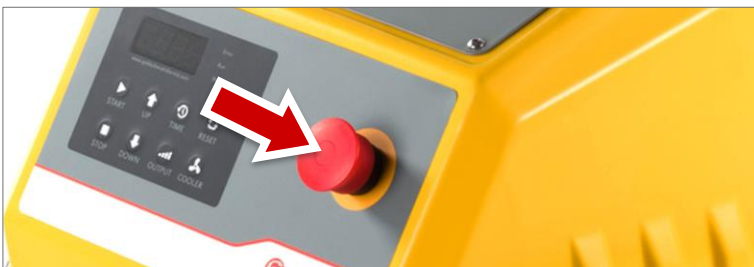
Figure 16: Emergency stop switch
