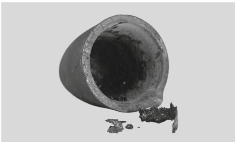
2. Removing the remainder with the slag bolt.
