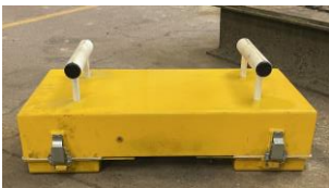
Figure 5: After use, place the Envirofilter™ on the floor, with the inlet facing down
