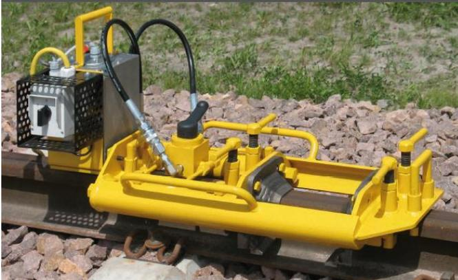
The shearing unit consists of a U-L 4 series shearing device and a series L power unit.
