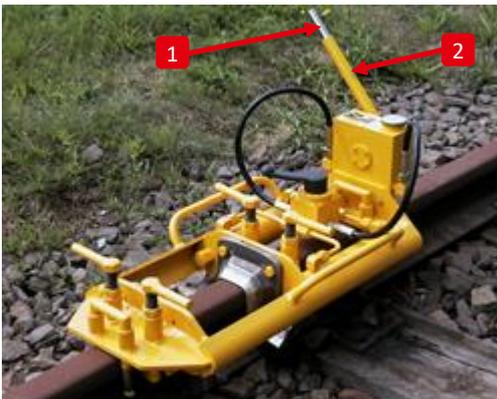
To shear, the extension (1) must be fitted on the stationary hand-operated lever (2) and this must be quickly moved back and forth. Approx. 25 to 30 double strokes are necessary depending on the welding process. Afterwards, it is advised to move it back quickly without the extension to protect the cutting edges.
