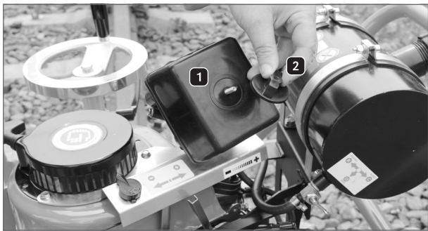
Figure 29: GP 4000 P – Check the air filter 1
