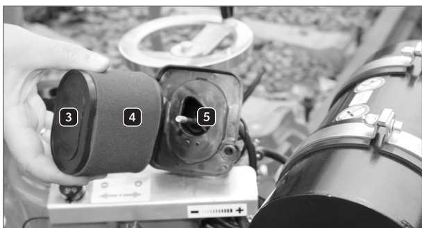
Figure 30: GP 4000 P – Check the air filter 2
