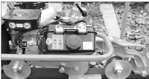
Figure 22: Oil fill plug for cold start
