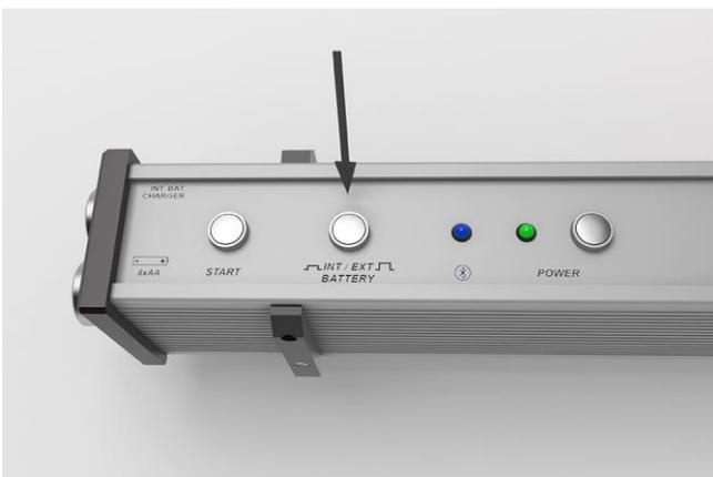
6. Press the **INT / EXT BATTERY** button on the Railstraight.
