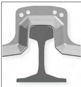
Fig. 2-2 Shear bladetype A - flat-bottom rails
