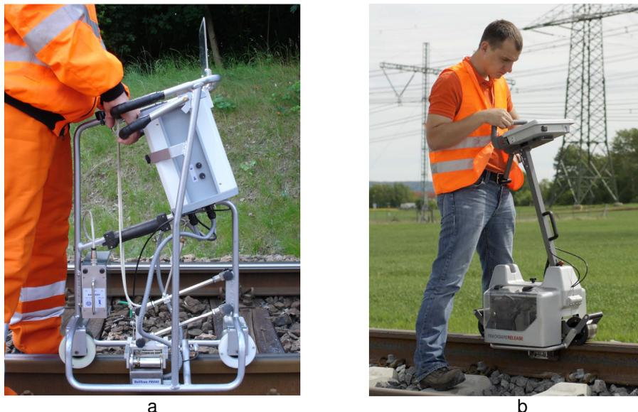
Fig. 3: Different RailScan and TRACKSAFE RELEASE device design generations. a: RailScan 2009-2011 during SFT inspections in Halle Germany, b: TRACKSAFE RELEASE 2012 after full redesign during trials on German High Speed Line Nürnberg – Berlin construction site near Erfurt.
