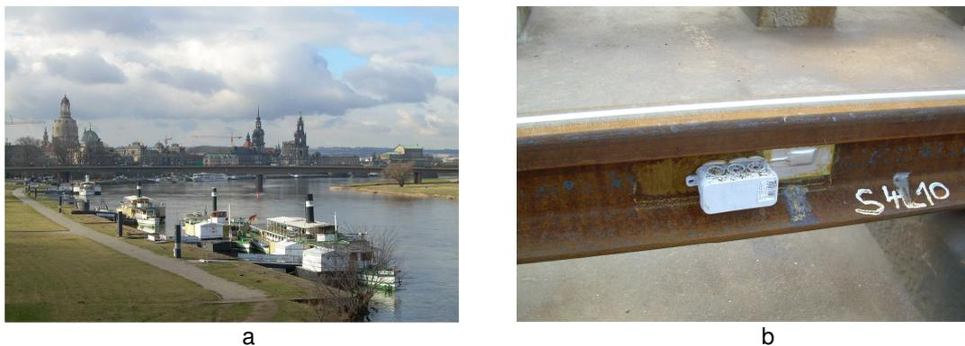
Fig. 6: Example of rail longitudinal stress monitoring. a: Site view of the monitored railway and road bridge across the Elbe. b: Applied strain gauge in bonding technique and completed weatherproof protection; The white box represents a protection for connection components.
