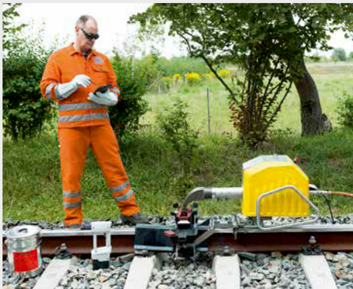
Left: Smartweld Jet is an automated propane/air preheating device.
