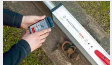
Right: Railstraight Dual is used for simultaneous measurement of the running surface and the gauge face.
